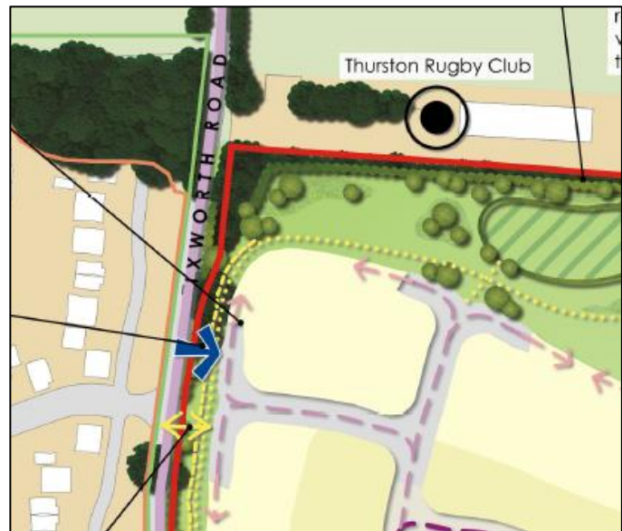
Figure 4: Indicative emergency vehicle access
